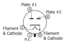
free pins not to be connected externally. generally pin 8 is used as cathode (output)
