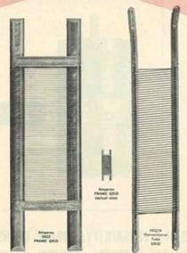
In the Amperex 6922 Frame Grid, note the fine wires under tension with the tight tolerances of the grid-to-cathode spacing determined by the carefully controlled diameter of the centerless ground grid-support rods and the frame cross-braces between these rods.
