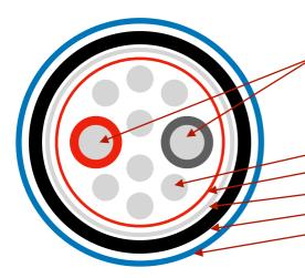
Central conductor: 2 conductors Copper OFC
