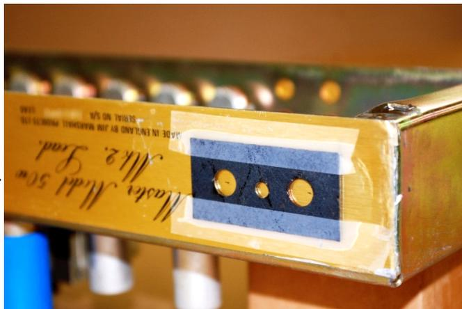
**Step 2: Drill it Out** Drill the holes with either a step bit or a regular metal cutting bit. Holes for the Send and Return should be 7/16" in diameter. The hole for the Bypass should be 3/16" in diameter.
